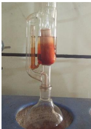
Figure 2: Soxhlet extraction of Areca catechu dye
