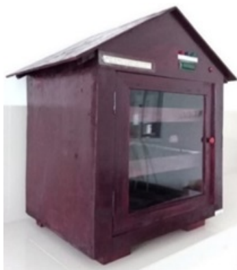
Figure 4: Smart Hybrid Drying chamber.
