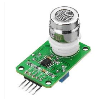
Fig 6: MG 811 Co 2 gas sensor.
