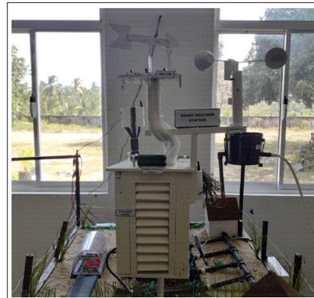
Fig 5: Smart weather monitoring system.
