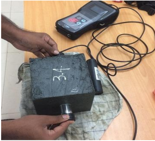
Figure 3: Pulse velocity measurement.
