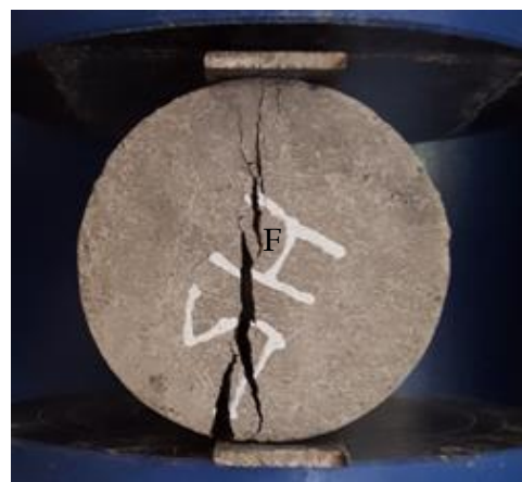
Figure 2: Splitting tensile loading.
